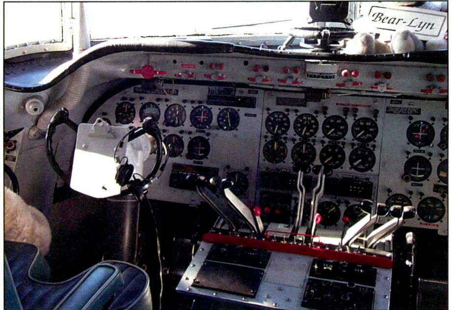
Airplanes were the first to adopt radio on a wide scale after ships, and the prevailing mode was AM. This older aircraft has new radios added to it which are just visible at the bottom of the center console.
