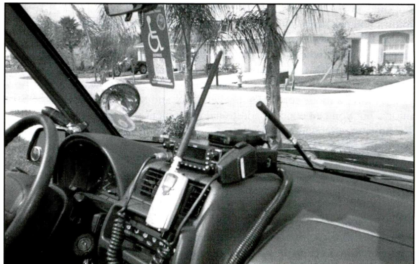
The low-profile LRD-767 mounted in a commo vehicle, among other telematic devices.
