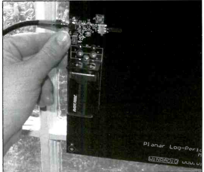
A small switch turns on the antenna, activating a small red LED.
