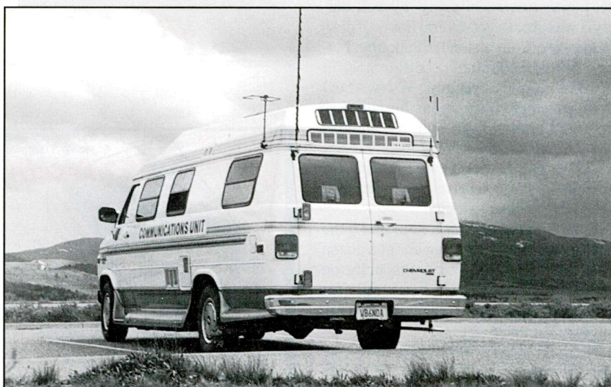
All antennas on Gordo's van are mounted up high and all are on lip mounts!
