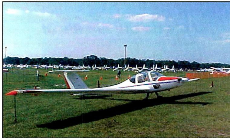
Here's a Europa Motor Glider — a glider that doesn't need a tow plane to get in the air.
