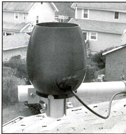
This sensor measures rainfall. It's mounted on my 2-meter antenna mast.
