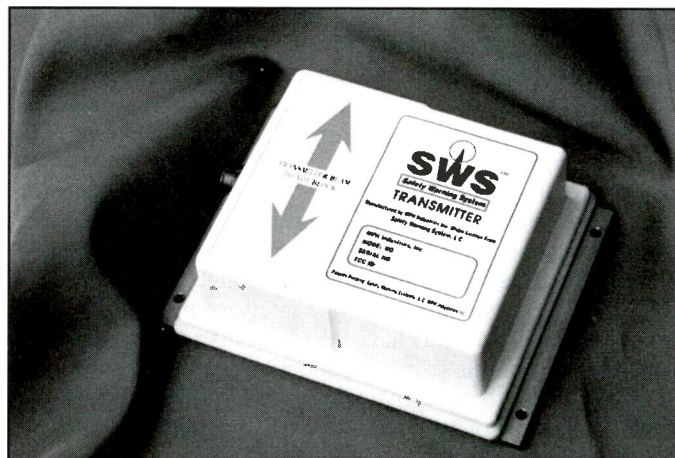
Safety Warning System transmitting unit.
